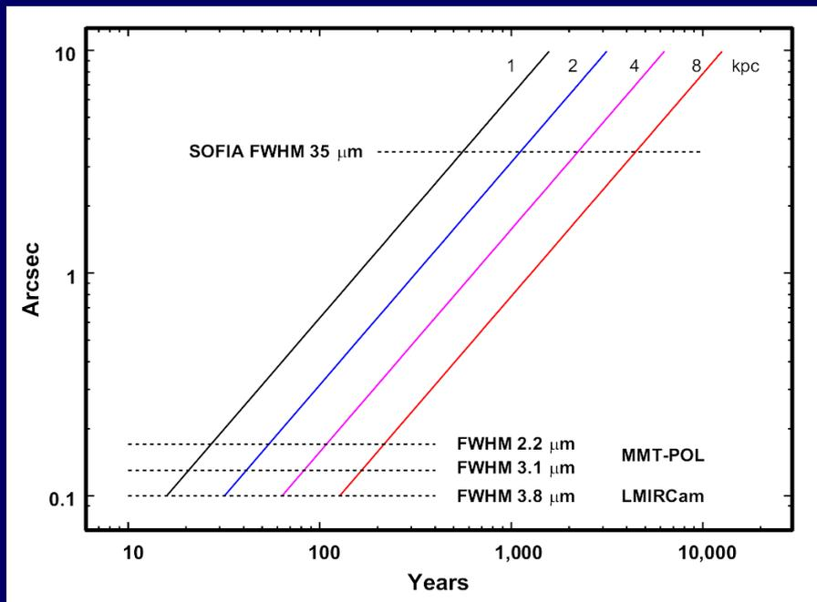
Relation between imaging resolution and travel time for dust in a 30 km/s wind.
